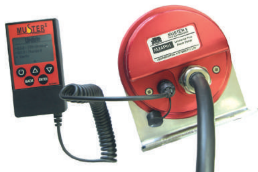
Diagnostic Module connected to Alarm Panel
